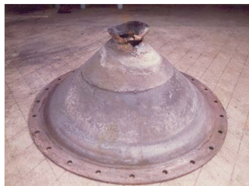
Fig. 2— (b) Damaged throat portion of Ankur gasifier.
